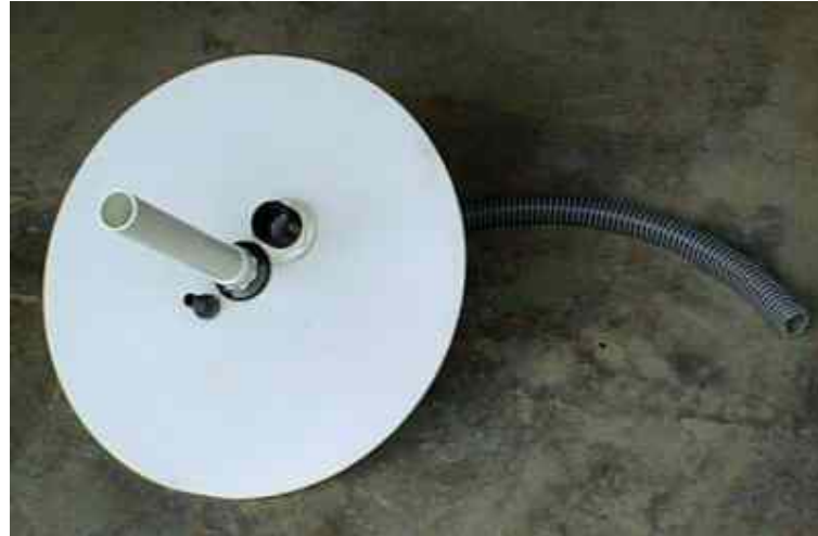
Assembled baffle plate ready for installation in tank.
